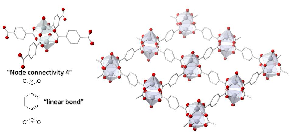
Metal centers with IC = 5 form dimers that generate a connectivity node 4 (SBU) and define a 2D coordination polymer with square windows.
