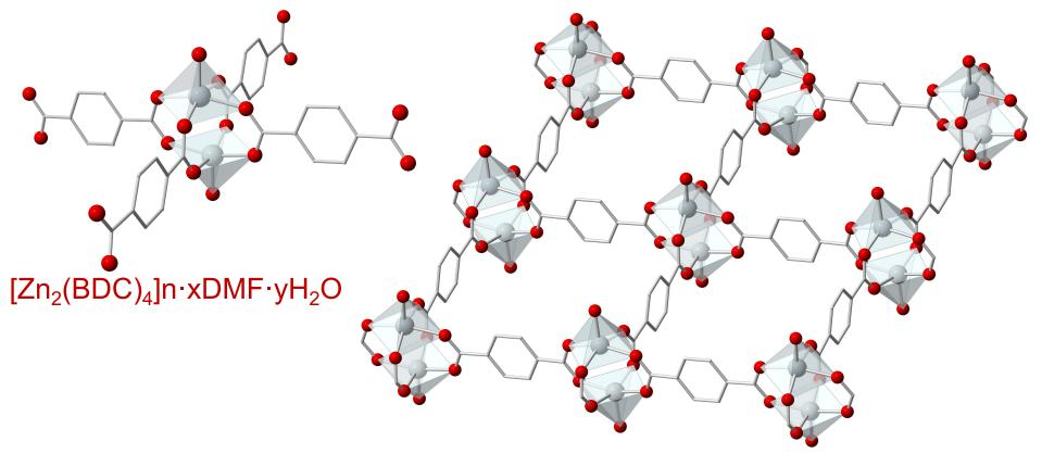
After removing the DMF and  $H_2O$  molecules included between the 2D layers the resulting formulated compound  $[Zn(BDC)_2]_n$  is thermally stable in the temperature range 190-315 °C
