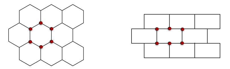
From a topological point of view there is no difference between a tetrahedron and a square. The regular connection of tetrahedral centres gives rise to a 3D network of the diamond type. But square connections give rise to a square 2D network. This is a difficulty in the description of the networks but in spite of that the topological analysis is very useful as demonstrated by A. F. Wells.
