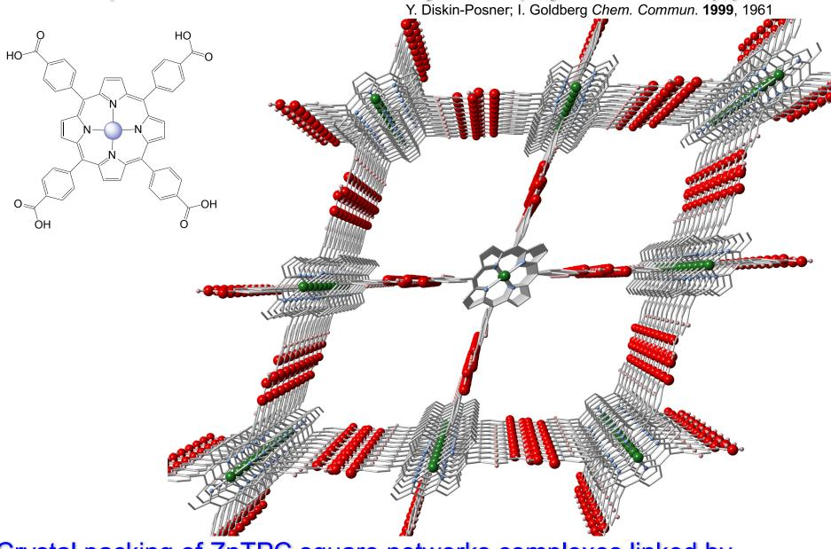
Crystal packing of ZnTPC square networks complexes linked by hydrogen bonds originates a CP with wide pores
