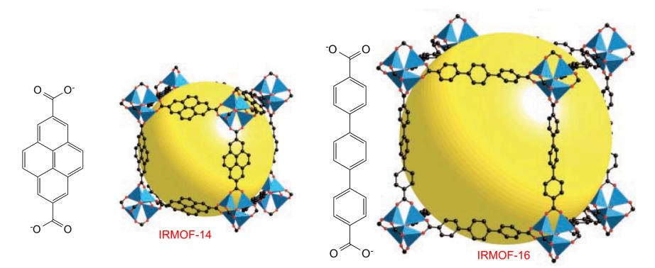
The members of this series with longer bridge ligands have pore sizes in the range of mesoporous materials (> 20 Å) and the lowest density observed for a crystalline material (so far, 2002). In particular IRMOF-6 presents the ability to adsorb  $CH_4$  to the greatest extent. During the preparation of this series the synthesis of MOF-5 was improved: Zn(NO<sub>3</sub>)<sub>2</sub>·4H<sub>2</sub>O + 1,4-benzenedicarboxylic acid (BDC) in DEF, heated (85°-105° C) in autoclave.
