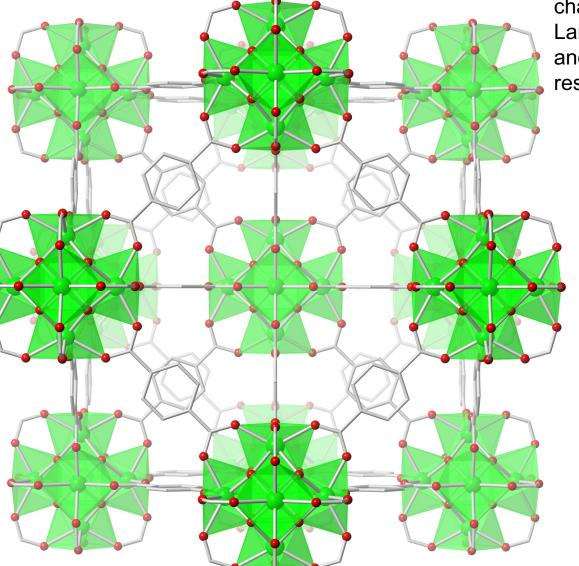
characterized by a  $T_{descp}$  = 540°C and Langmuir surface 1187m<sup>2</sup>/g, 3000 m<sup>2</sup>/g and 4170 m<sup>2</sup>/g for UiO-66, -67 and -68, respectively
