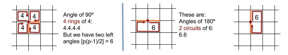
The Vertex Symbol for this 2D layer is: 4.4.4.\*.\* since VS does not consider circuits. The two asterisks are added to be consistent with p(p-1)/2. It is important to note that the VS does not explicitly contain the connectivity of the nodes, it only specifies the poligonality. However, the value p(p-1)/2 is the sum of the "exponents" of the corresponding symbols (including asterisks).
